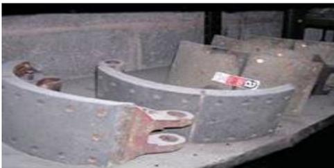
Asbestos containing friction products. e.g. conveyor and fan belts, brake and clutch linings (non-friable)
