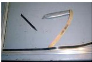
Asbestos containing mastics around windows, wall expansion joints, joints in HVAC ductwork (non-friable)
